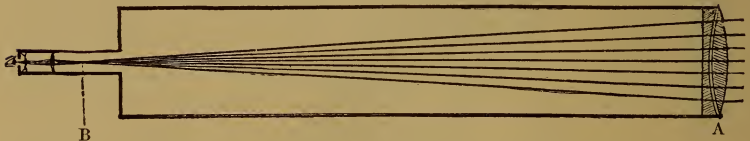
FIG. 86.—ILLUSTRATION OF THE PRINCIPLE OF REFRACTORS.
